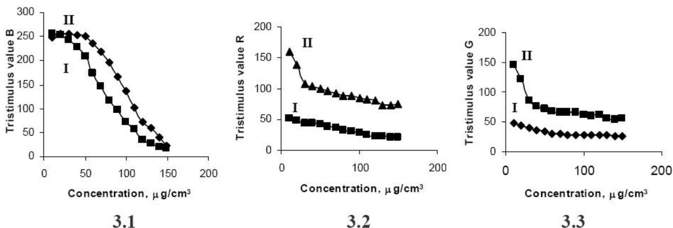
**Figure 3:** Influence of the light source intensity to the graph curve of tristimulus value against solution concentration. 3.1- for tristimulus value of B. 3.2- for tristimulus value of R and 3.3- for tristimulus value of G. I-for less intense light source and II-for more intense light source.
